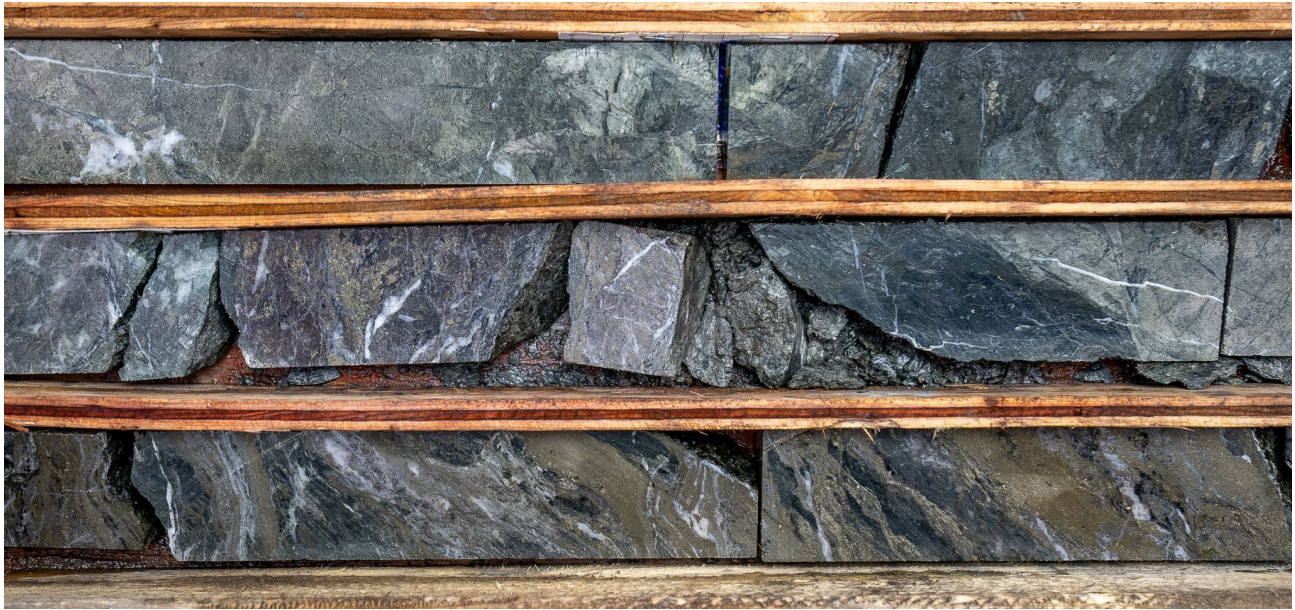
Figure 2: Drill core from hole SR20-27 – Textural example of high-grade gold mineralization present within the O-zone – sections of the core sample above graded 109.4 g/t gold and 32.4 g/t silver over 2.53 metres. Throughout the interval intense chlorite alteration has destroyed original textures in the host andesite, minor patchy sericite occurs along shear surfaces, and quartz-carbonate veining and alteration are present throughout the interval. Sulphides (20% pyrite, 8% pyrrhotite, 0.1% galena) are blebby, or occur in elongate lenses that are generally aligned with shear fabric. Zones of semi-massive sulphide (lower row), contain ~ 45% pyrite, 20% pyrrhotite, and have been subjected to intense shearing. For scale, drill core is approximately 50 mm in diameter.
