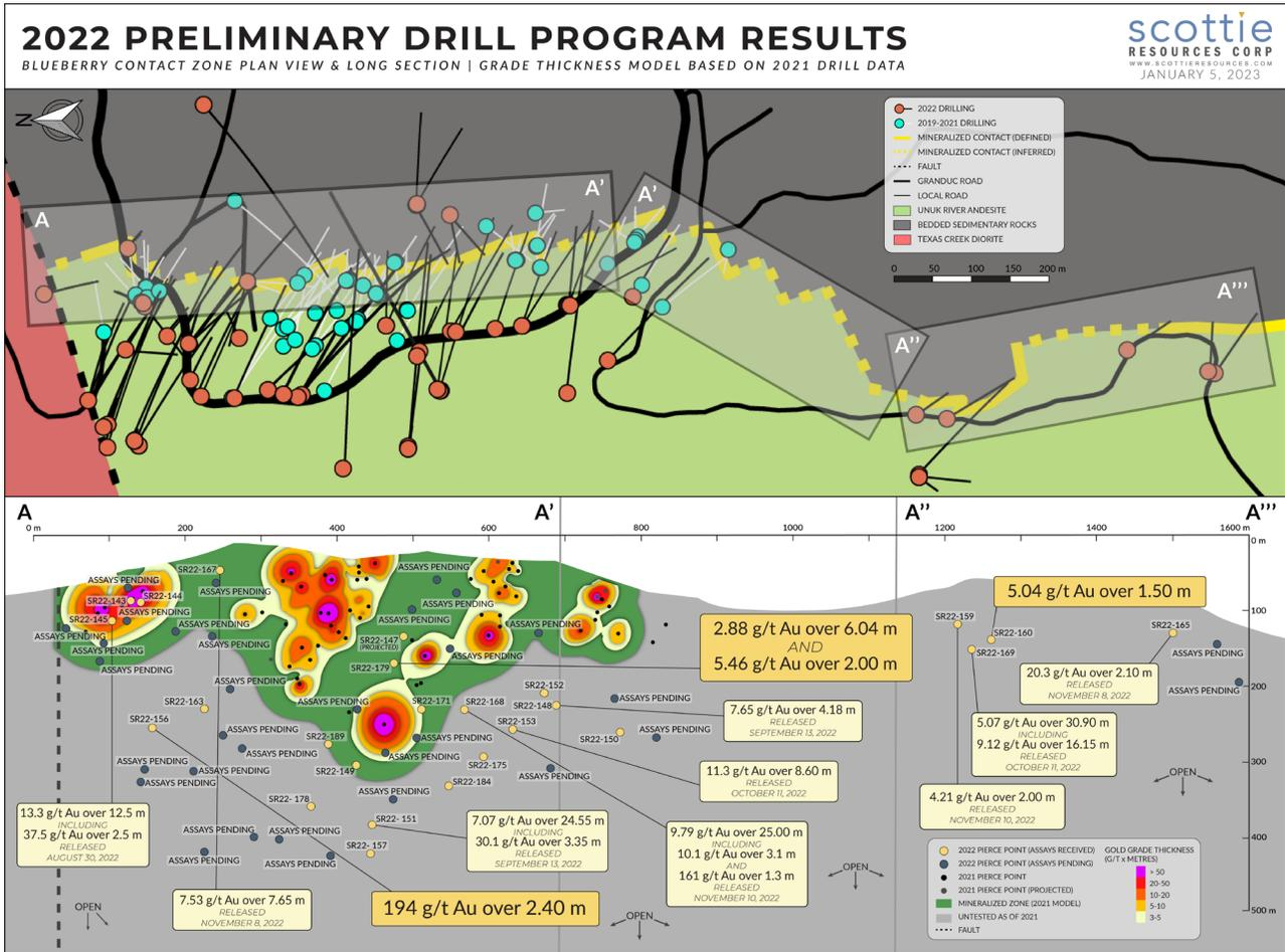
**Figure 1:** Segmented vertical long section of the Blueberry Contact Zone and plan view illustrating the distribution of the sections. Highlighting the distribution and status of drilled targets from the 2022 season and the reported results thus far, grade contour model was created from pre-2022 drilling of the structure.
