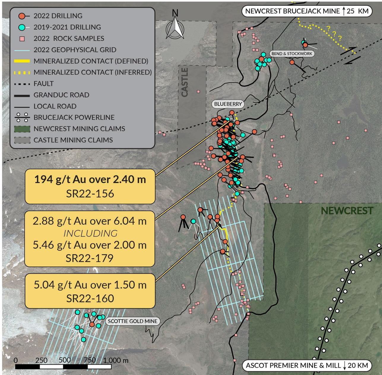
**Figure 2:** Overview plan view map of the Scottie Gold Mine Project, illustrating the distribution of the most recent results, and the overall scope of the 2022 drill and the completed 2022 loop electromagnetic geophysical grids.
