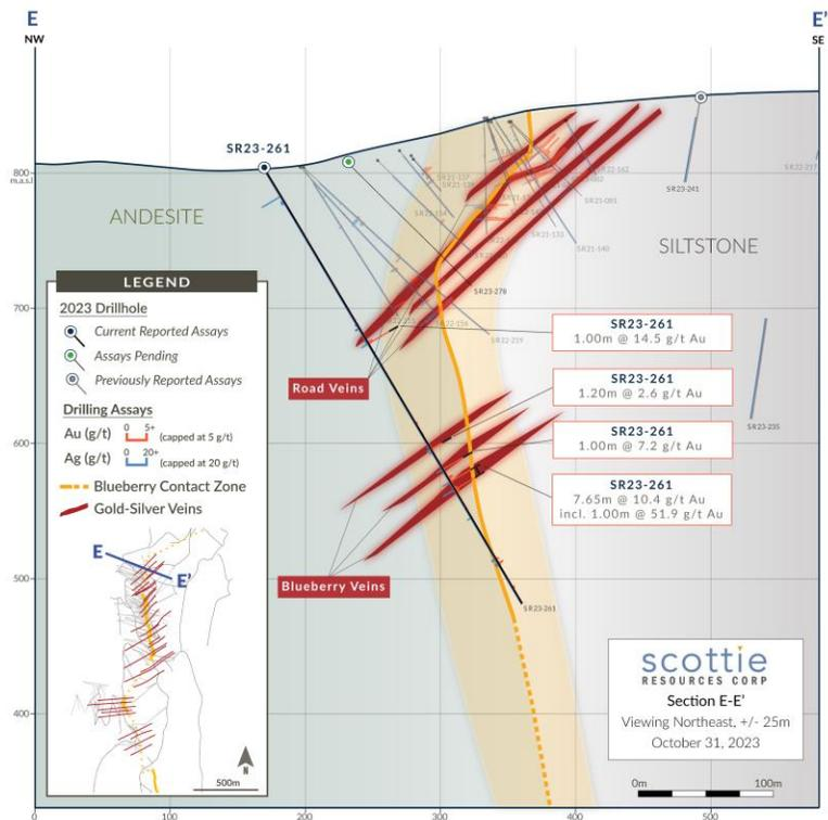
**Figure 2:** Cross-section displaying vein and contact style intercepts highlighted by the recent intercept in SR23-261 located in the Road vein portion of the Blueberry Contact Zone.
