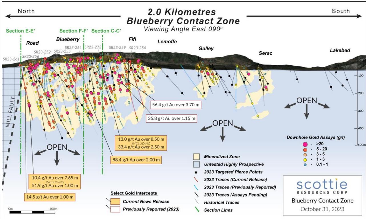
**Figure 5:** Segmented vertical long section of the Blueberry Contact Zone illustrating the distribution and status of drilled targets from the 2023 season and the reported results thus far, relative to intercepts from previous drilling campaigns.
