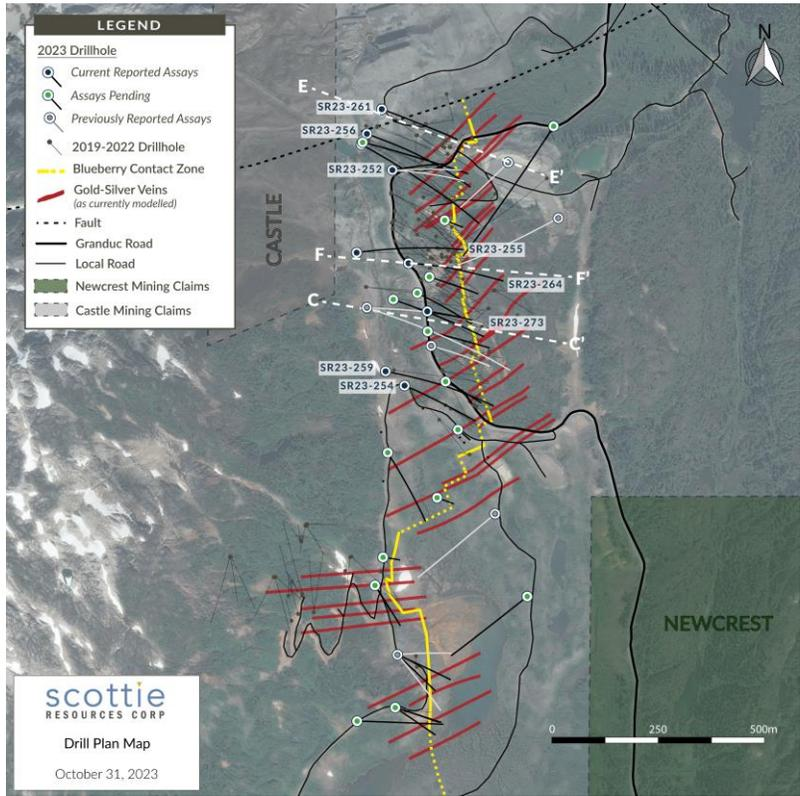
**Figure 1:** Overview plan view map of the Scottie Gold Mine Project, illustrating the locations of the reported drill results, cross-sections (Figures 2 - 4), and the distribution of the modelled sulphide-rich cross-structures.
