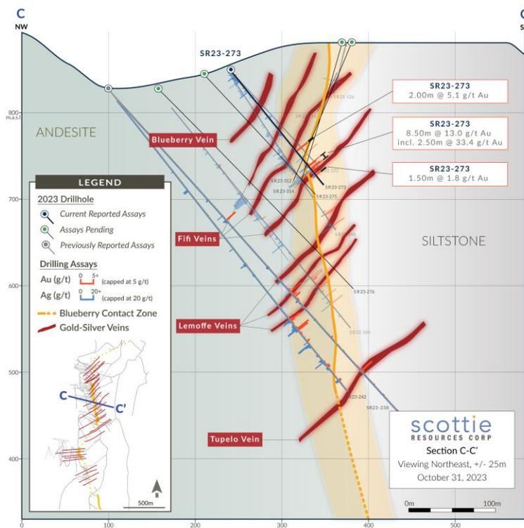
**Figure 4:** Cross section displaying vein intercepts highlighted by SR23-273 in the Fifi - Lemoffe portion of the Blueberry Contact Zone. Cross-section is updated from the original C – C’ section released on [September 6, 2023](#).
