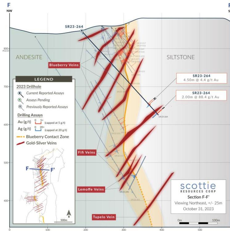
**Figure 3:** Cross-section displaying vein intercepts highlighted by SR23-264 in the Fifi - Lemoffe portion of the Blueberry Contact Zone.
