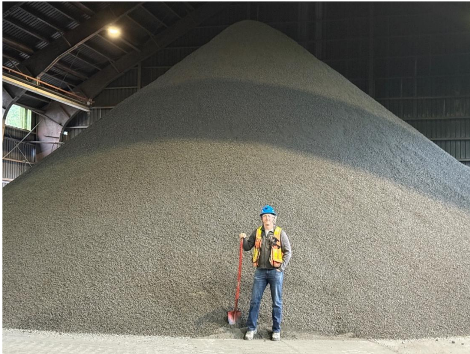
Figure 2 - Photo of Bulk Sample at Stewart Bulk Terminal awaiting transport. Product has been crushed to ½" minus. Scottie COO Sean Masse for scale.
